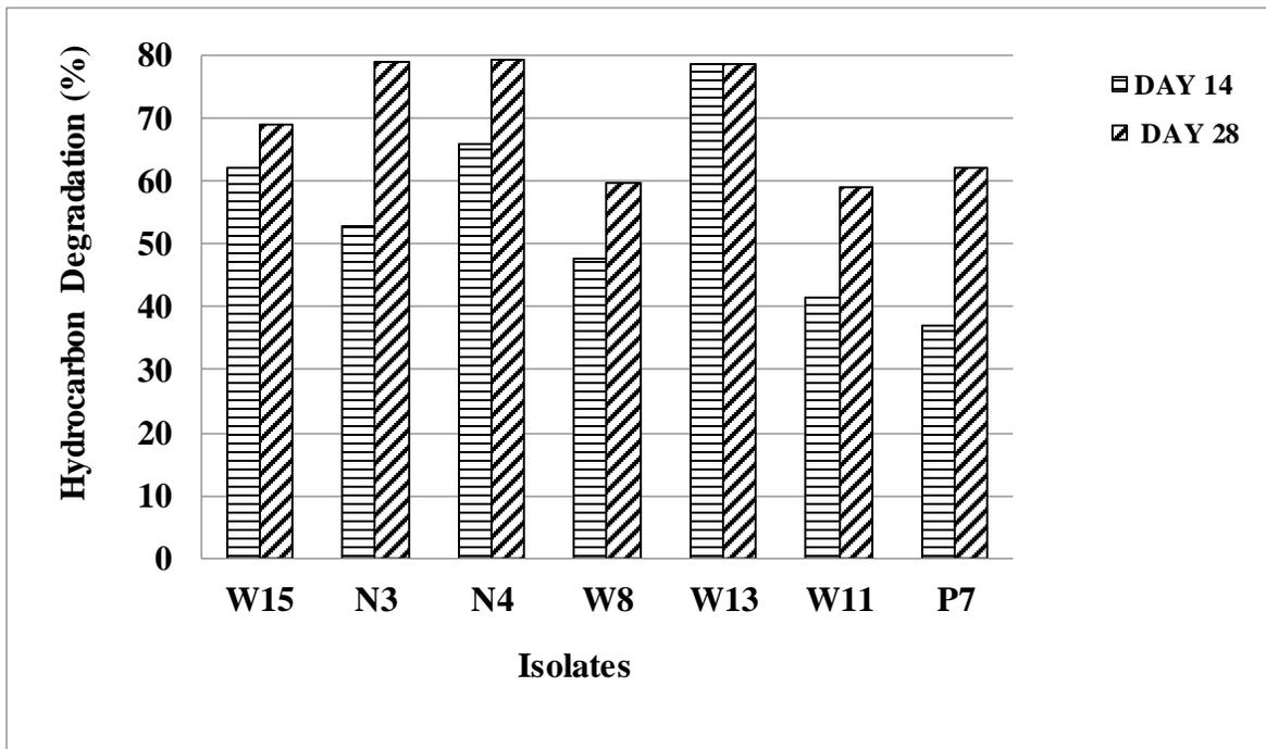
**Figure 5:** Percentage total petroleum hydrocarbon degraded by the isolates at Day 14 and Day 28 of incubation
