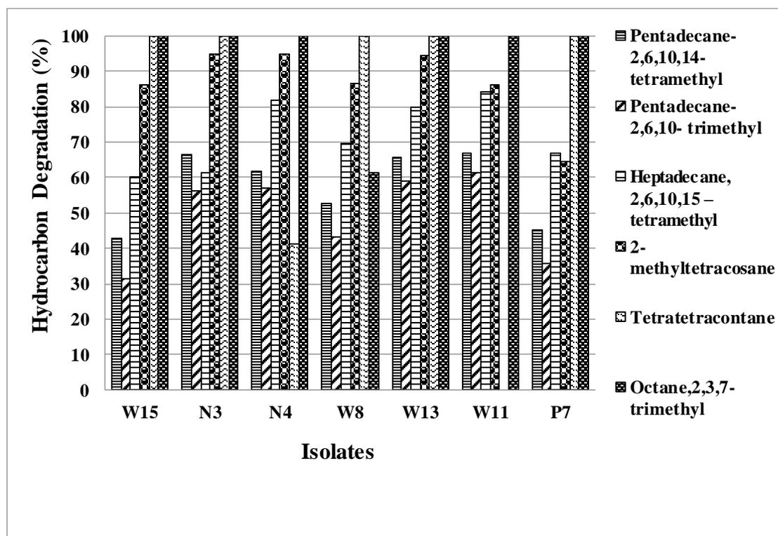
**Figure 6:** Percentage degradation of alkane fractions by single isolates after the 28 days of incubation
