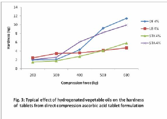
Fig. 3: Typical effect of hydrogenated vegetable oils on the hardness of tablets from direct compression ascorbic acid tablet formulation
