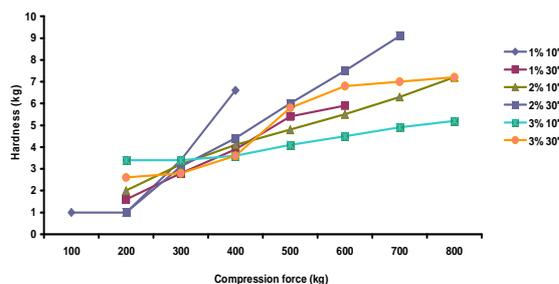
Fig 5: Effect of Lubritab concentration and mixing time on the hardness of ascorbic acid tablets
