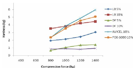
Fig 6: Typical effect of named excipients on the hardness of tablets compressed from a direct compression acetaminophen tablet formulation
