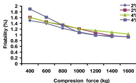
Fig 8: Effect of STX concentration and mixing time on the friability of tablets compressed from the model direct compression formulation
