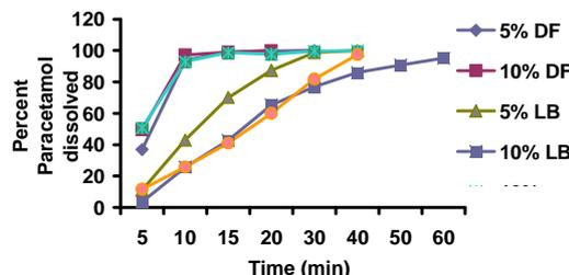
Fig 10: Typical effect of excipients on paracetamol dissolution from aspirin-paracetamol tablets
