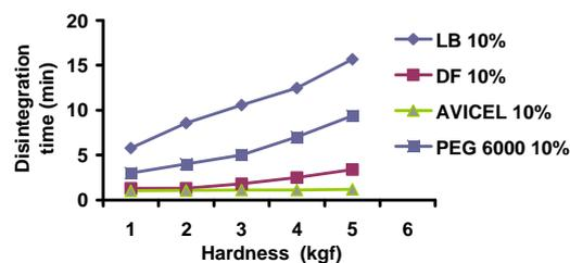
Fig 9: Typical effect of excipients on the disintegration time of tablets compressed from a direct compression hydrochlorothiazide tablet formulation
