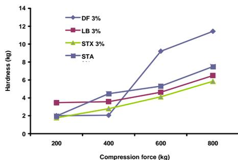
Fig. 4: Typical effect of hydrogenated vegetable oils on the hardness of a direct compression ascorbic acid tablet formulation
