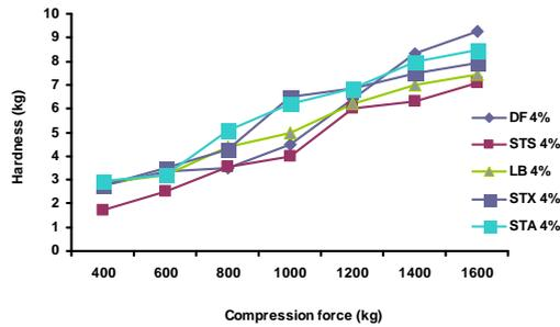
Fig. 1: Typical effect of hydrogenated vegetable oils on the hardness of tablets from a model direct compression tablet formulation
