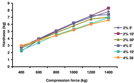
Fig. 2: Effect of Lubritab concentration and mixing time on the hardness of tablets from the model direct compression tablet formulation
