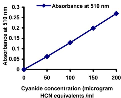
**Fig. 1: Calibration curve for cyanide determination by the alkaline picrate method**
